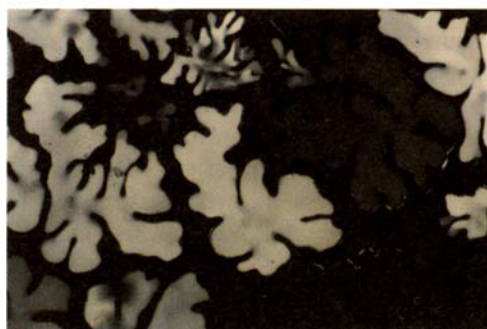
Figure 6. Optical photomicrograph of the texture observed at the transition from the smectic A phase (homeotropically oriented sample between crossed polarizers) to the low temperature mesophase of compound 5 at 173°C.
